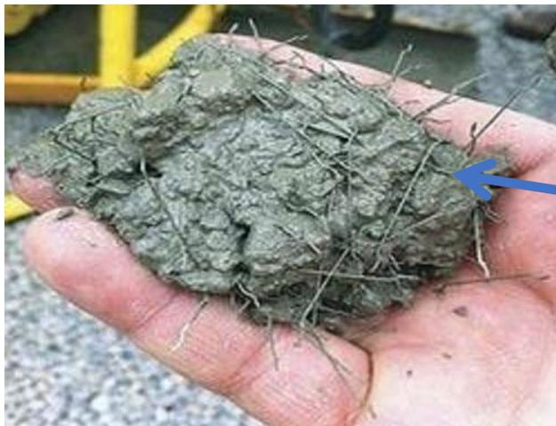
Concrete with Steel Fibres
